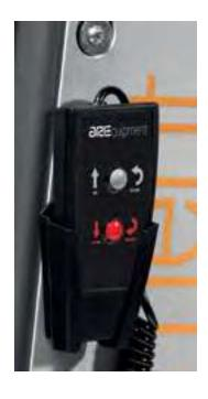
MOVEMENTS: (1-A) Platform opening: keep button 1 pressed until the complete platform opening, which stops at the same level as the vehicle floor automatically. (1-B) Repeat the previous operation, press button 1 until the platform reaches the ground. (2-A) Press button 2 to lift the platform to reach the same level as the vehicle floor. (2-B) Then press button 2 again and keep it pressed until the complete platform closing.
