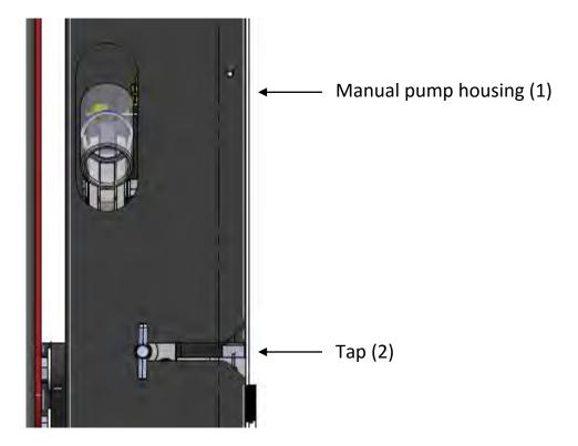
The manual pump and the tap allow a usage of the lift in case of electric system failure.
