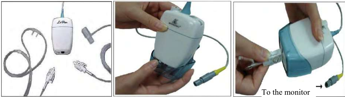
Fig 16-3 Respiroics Sidestream CO 2 Connection Diagram
