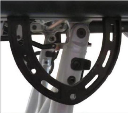
U-profile with removed side loading wheel
