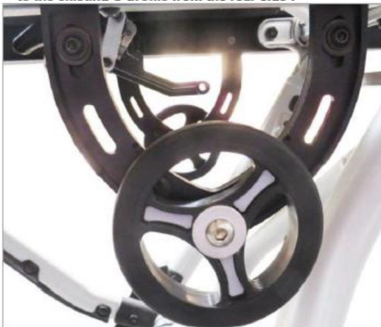
Fixed additional U-profile with mounted loading wheel
