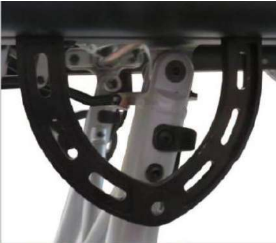
U-profile with removed side loading wheel
