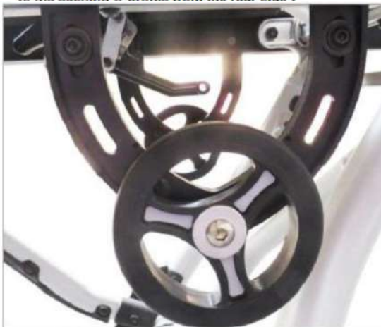
Fixed additional U-profile with mounted loading wheel
